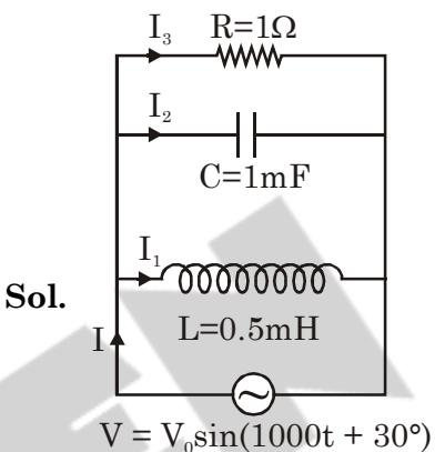
$$R = 1\Omega, x_C = \frac{1}{\omega C} = 1\Omega, X_L = \omega L = 0.5$$
