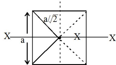
XX is in axis of symmetry so centre of mass lie on XX at centroid position of dotted triangle.
