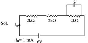
Pot. Diff. across each resistor = 2V q = CV =  $50 \times 10^{-6} \times 2 = 100 \times 10^{-6} = 100 \ \mu C$
