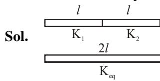
$$R_{\text{eff}} = \frac{l}{K_1 A} + \frac{l}{K_2 A} = \frac{2l}{K_{\text{eq}} A}$$
