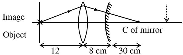
For the object to coincide with image, the light must fall perpendicularly to mirror. Which means that the light will have to converge at C of mirror.
