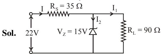
$$\text{Voltage across } R_S = 22 - 15 = 7 \text{ V}$$
