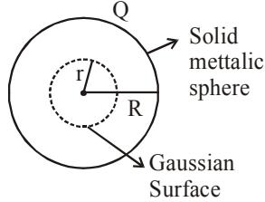
As change encloses within gaussian surface is equal to zero.
