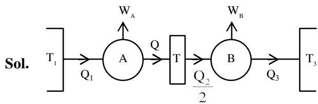
$$W_A = 1 - \frac{Q_2}{Q_1} = 1 - \frac{T}{T_1} \Rightarrow \frac{Q_2}{Q_1} = \frac{T}{T_1}$$
