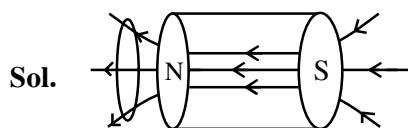
→ When magnet passes through centre region of solenoid , no current / Emf is induced in loop.
