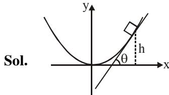
At maximum ht. block will experience maximum friction force. Therefore if at this height slope of the tangent is  $\tan \theta$ , then  $\theta$  = Angle of repose.
