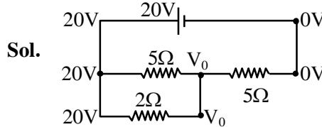
$$\frac{20 - V_0}{5} + \frac{0 - V_0}{5} + \frac{20 - V_0}{2} = 0$$
