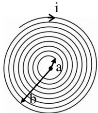
$$\text{No. of turns in } dx \text{ width} = \frac{N}{b-a} dx$$
