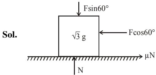
$$F \cos 60^\circ = \mu N \text{ or } \frac{F}{2} = \frac{1}{3\sqrt{3}}N \quad \dots (1)$$
