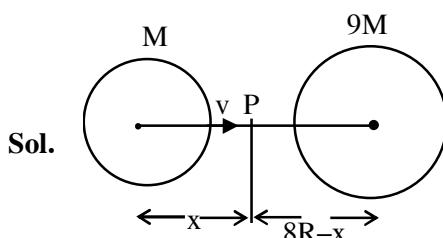
Acceleration due to gravity will be zero at P therefore,
