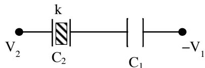
$$Q = \left[ \frac{C_1 C_2}{C_1 + C_2} \right] [V_1 + V_2]$$
