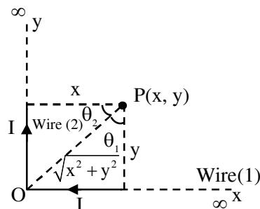
$$B_{\text{due to wire (1)}} = \frac{\mu_0 I}{4\pi y} [\sin 90^\circ + \sin \theta_1]$$
