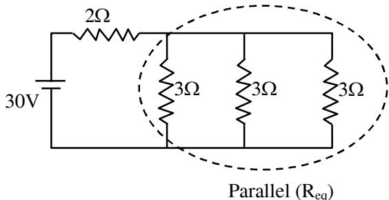
$$\frac{1}{R_{eq}} = \frac{1}{3} + \frac{1}{3} + \frac{1}{3} = 1 \Rightarrow R_{eq} = 1\Omega$$
