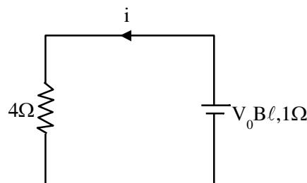
$$i = \frac{V_0 B \ell}{4+1} \Rightarrow V_0 = \frac{5(2\text{mA})}{5 \times 2} = 10^{-2} \text{ m/s} = 1 \text{ cm/s}$$
