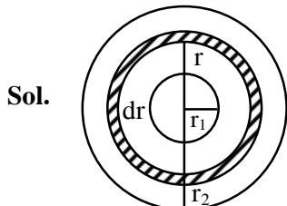
Thermal resistance of spherical sheet of thickness  $dr$  and radius  $r$  is
