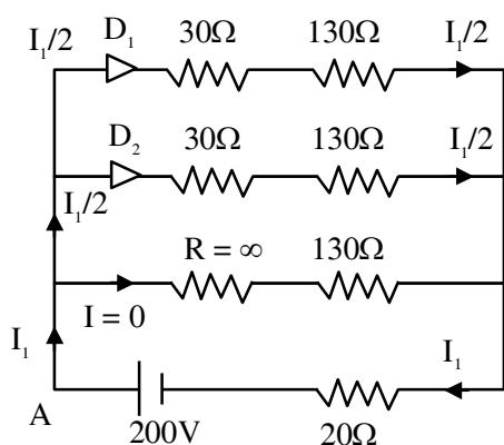
$$-\left(\frac{I_1}{2}\right) \times 30 - \left(\frac{I_1}{2}\right) \times 130 - I_1 \times 20 + 200 = 0$$
