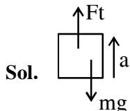
$$F_{\text{thrust}} = \left( \frac{dm}{dt} \cdot V_{\text{rel}} \right)$$
