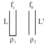
$$L' = \frac{4L}{3} \frac{V_0}{V_C} = \frac{4L}{3} \sqrt{\frac{B \cdot \rho_1}{\rho_2 \cdot B}} \quad (B \text{ is bulk modulus})$$
