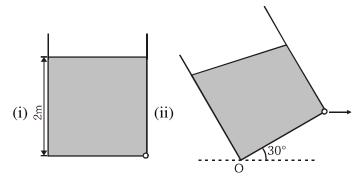
25. Liquid is filled in a vessel of square base  $(2m \times 2m)$  upto a height of 2m as shown in figure (i). In figure (ii) the vessel is tilted from horizontal at 30°. What is the velocity of efflux in this case. Liquid does not spills out?
