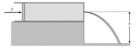
23. With what velocity the liquid comes out of the orifice?
