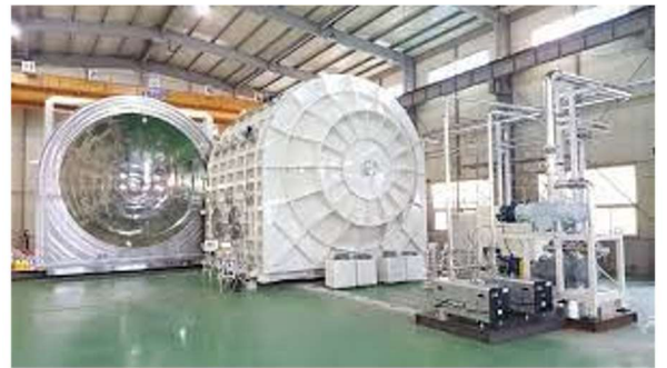
Figure: Dirty Thermal Vacuum Chamber
